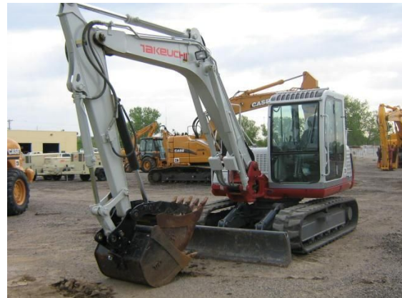
8 ton Takeuchi excavator
